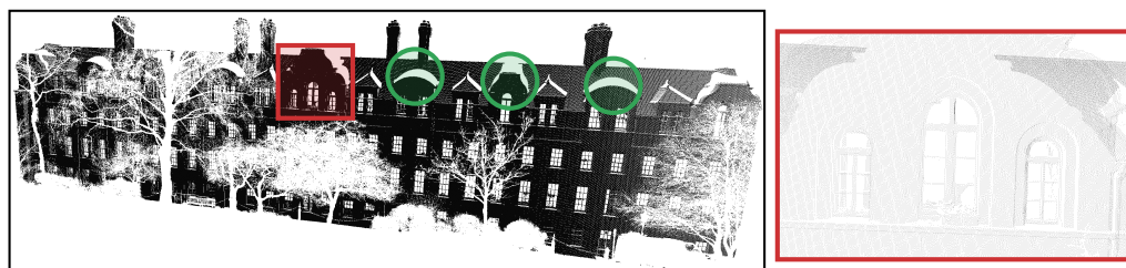
Figure 2.10: TLS points acquired on a building from a single scanner position. The inset (red rectangle) shows a close-up view where it is possible to identify individual points and small features, such as window frames. Green circles show three regions where raised windows occlude roof parts.
