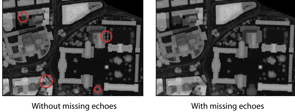
Figure 15.8: Left : Pixels in an elevation image to which no points map are black and dark regions correspond to areas where no points are available (red circles). Right : The insertion of missing echoes increases the availability of point data, thus reducing dark regions caused by an absence of information. In both elevation images pixel dimensions in global coordinates are: \Delta x_w = \Delta y_w = 0.2 \text{ m} .
