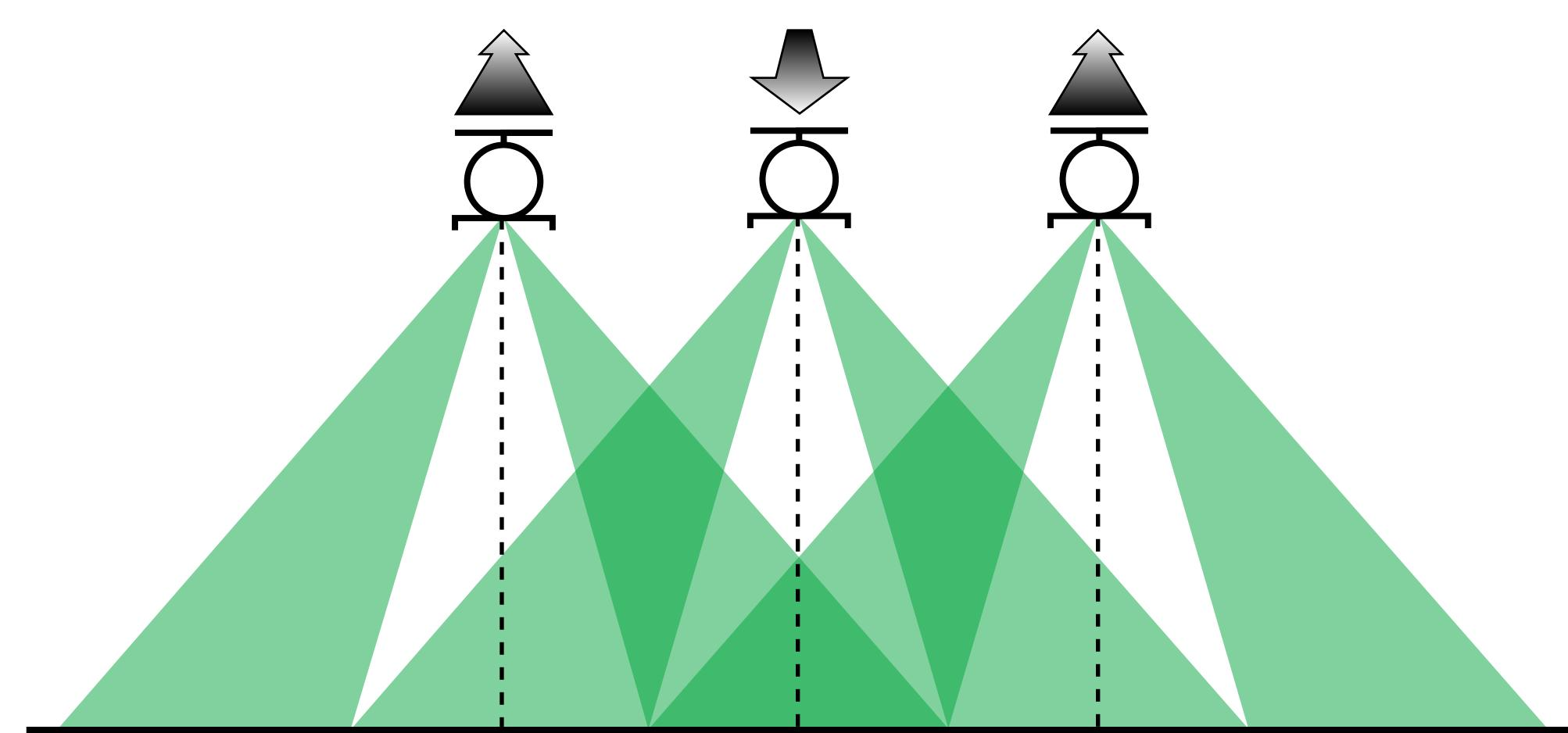
Full reliable coverage is achieved by a cross-pattern of triple overlapped flight tracks, with a little extra overlap to compensate for errors.
