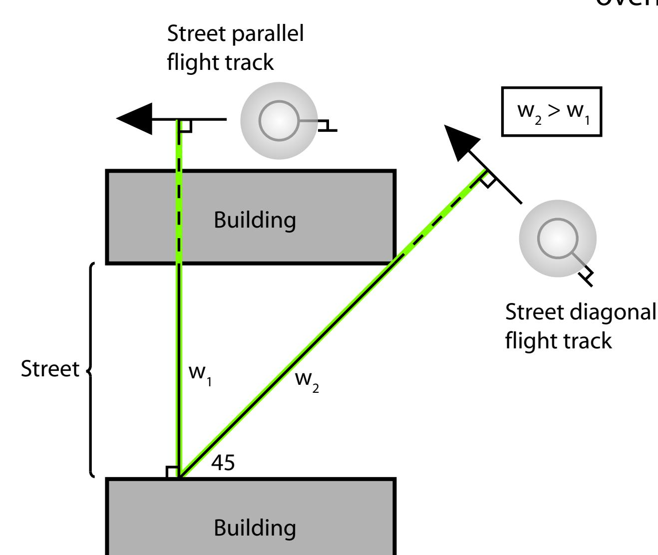
Flight tracks are aligned as much as possible at 45 degree angles to streets in order to avoid scanning building walls directly beneath the scanner.
