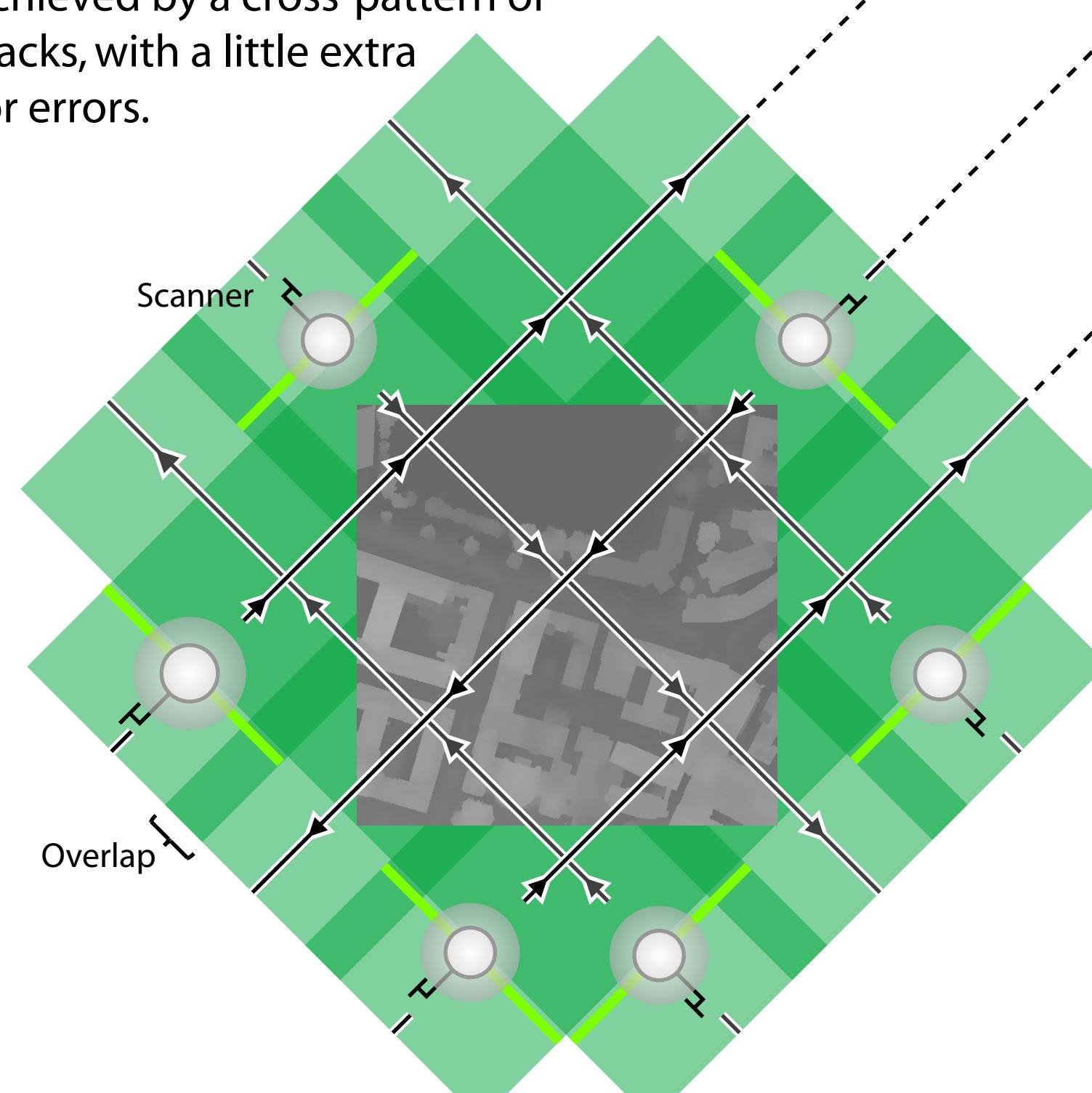
$$\text{Analytical scan quality: } R_H = h \sin \theta_L \sec^2 \theta_H \quad [\text{m}^2/\text{point}]$$
